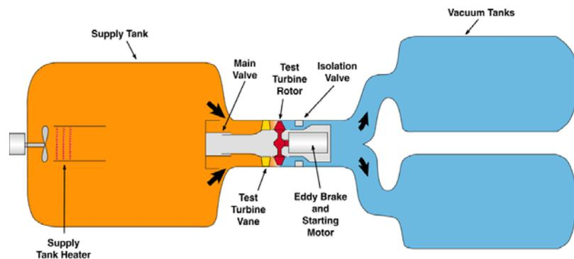
Figure 3 Block diagram of the Turbine Research Facility.
