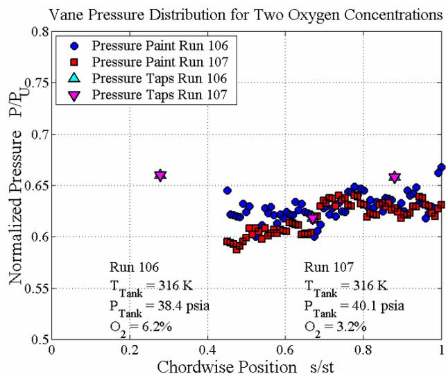
Figure 6 Normalized pressure near 50% span for two  $O_2$  concentrations.
