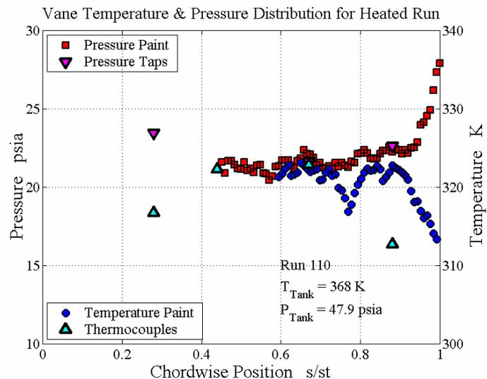
Figure 8 Pressure measurements at 50% span at elevated temperature.
