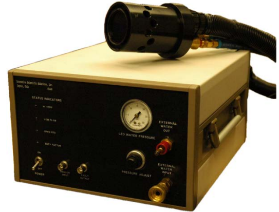
Components: LED head, umbilical, and control box.
