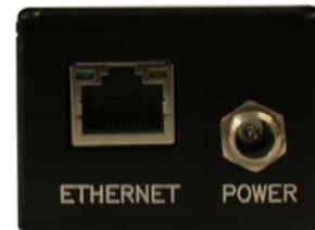
Ethernet / Power Connection
