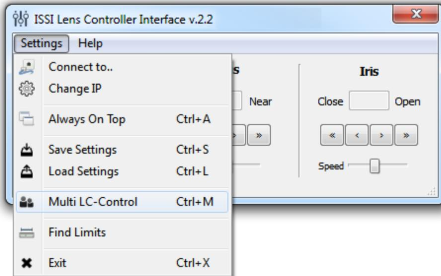
Before using the lens controller with a lens, the limits of the motors can be found using the **Find Limits** tool. For lenses with preset capability, this determines the minimum and maximum motor positions. The motors of the lens will move through their minimum and maximum points to establish the limits.
