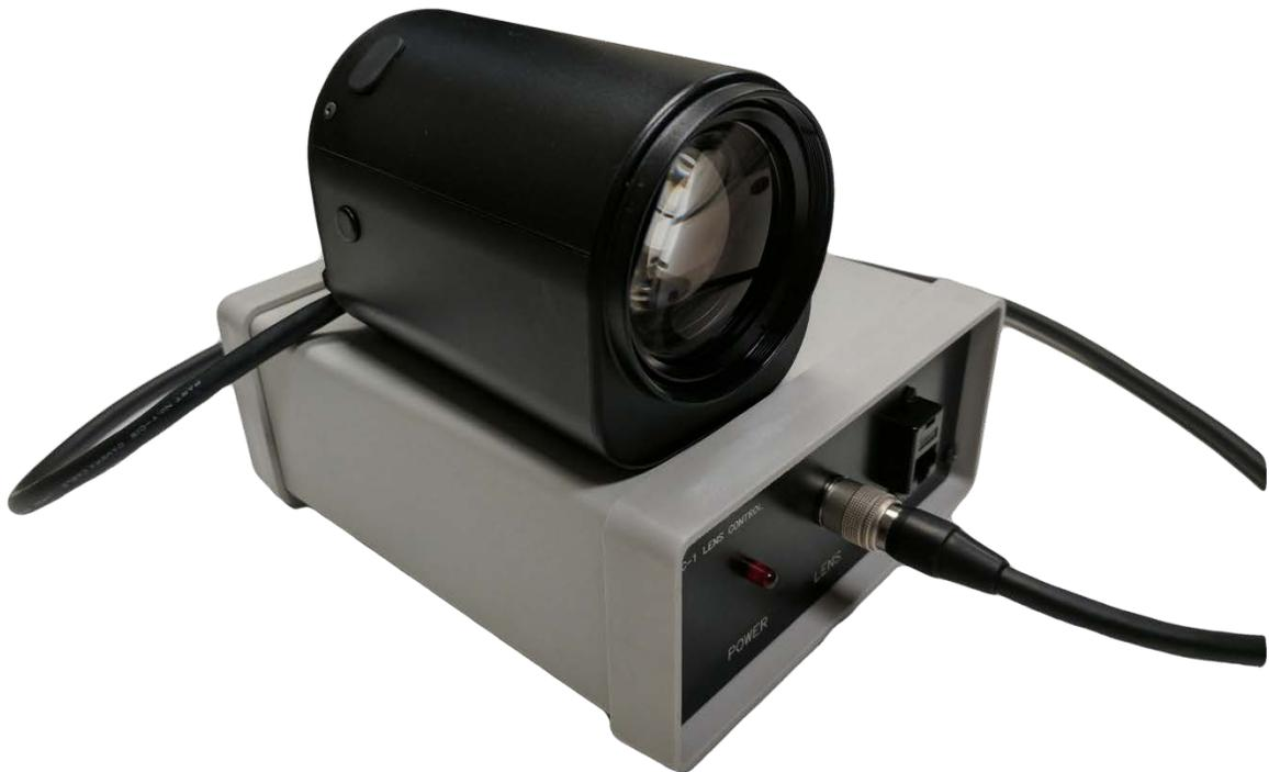
Use a Cat5 or Cat6 Ethernet cable (provided) to connect to a PC network interface card or network switch. The LC-1 is set up for universal power. The lens is supplied with a Hirose connection to connect to the LC-1. This is a keyed connection and will only attach one way. For users wishing to connect a specific lens other than that provided by ISSI, the connection pin-out is described on page 12.
