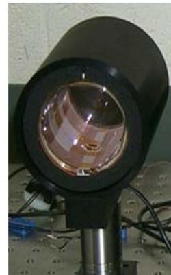
Packaged I2S-5 with integrated thermocouple and heating element in aluminum housing.
