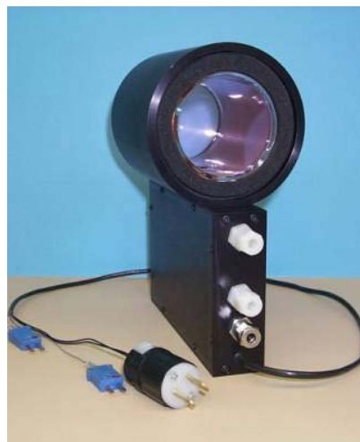
Packaged I2M-10 with thermocouples and heater.
