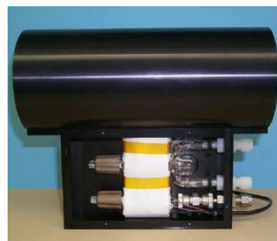
Side view of I2M-10 cell design.
