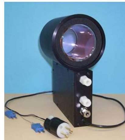
Packaged I2M-10 with thermocouples and heater
