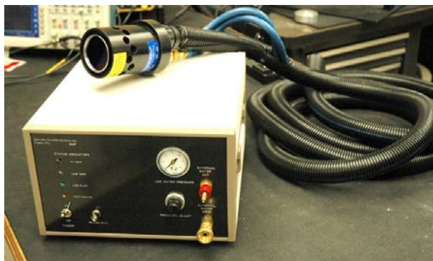
LM2XX-DM components: LED head, umbilical, and control box.
